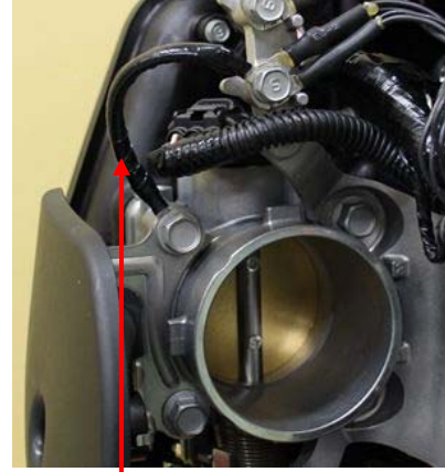
Extension wire lead attached
